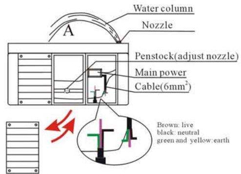
STEP2: connect the main power box to power
