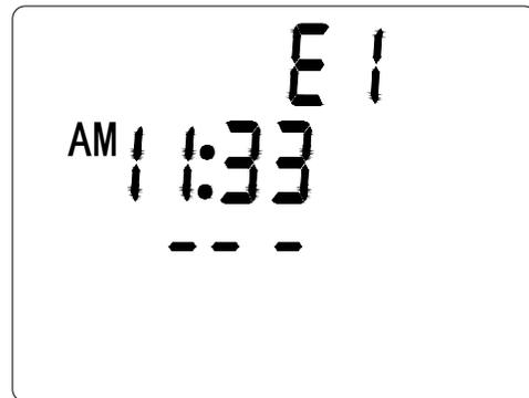
Fig . 4: Sensor open circuit or short circuit
