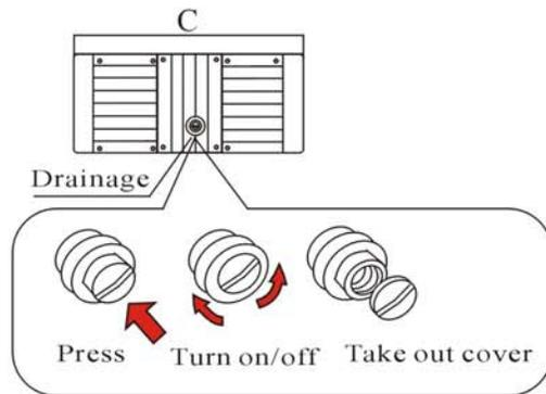
STEP4: install the drainage
