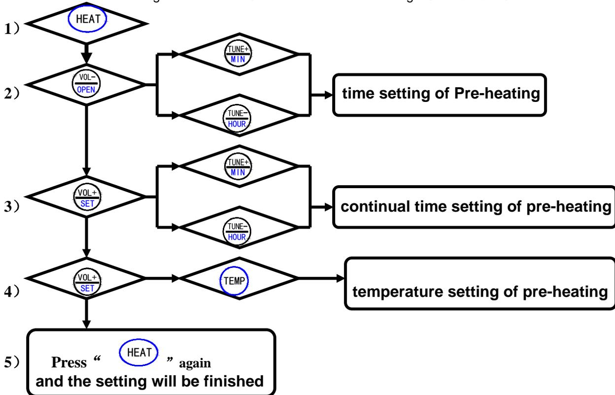
Pre-heating setting is in the “Power off” status and the LCD display “---”.
